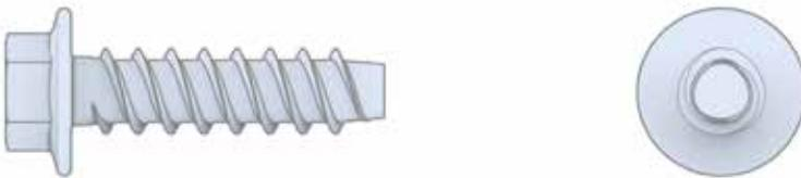
**PLASTITE® 48-2™** TRILOBULAR® thread-rolling screws have twin-lead threads to provide faster, more efficient insertion in plastic materials. The sharp 48° thread profile increases holding strength and reduces material displacement and boss bursting tendencies. Drive and strip torques are higher, making drive tool adjustments simple.
