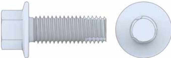
The **KLEERLOK®** feature is designed to be used in conjunction with TRILOBULAR® fasteners in pretapped holes which may be contaminated with weld splatter, paint, primer or other foreign matter.
