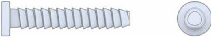
The **PUSHTITE® II™** fastener assembly process is accomplished by a simple press-in operation, reducing assembly time and simplifying serviceability. The PUSHTITE® II™ fastener's locking grooves are helical, allowing easy removal and reinsertion as necessary.
