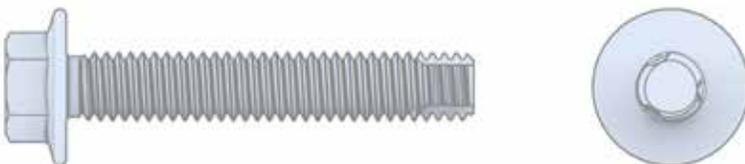
**KLEERTITE®** fasteners are a debris-clearing TRILOBULAR® screw for joints where a locking screw is not desired. Like their KLEERLOK® cousins, KLEERTITE® fasteners have the same ability to clear threads in pre-tapped holes contaminated with weld splatter, paint, primer or other foreign matter.
