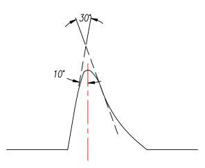
The REMFORM® II™ "HS" unique asymmetrical radius flank thread form has the thread forming advantages of a 30° thread, without the difficulty of manufacturing a 30° thread.
